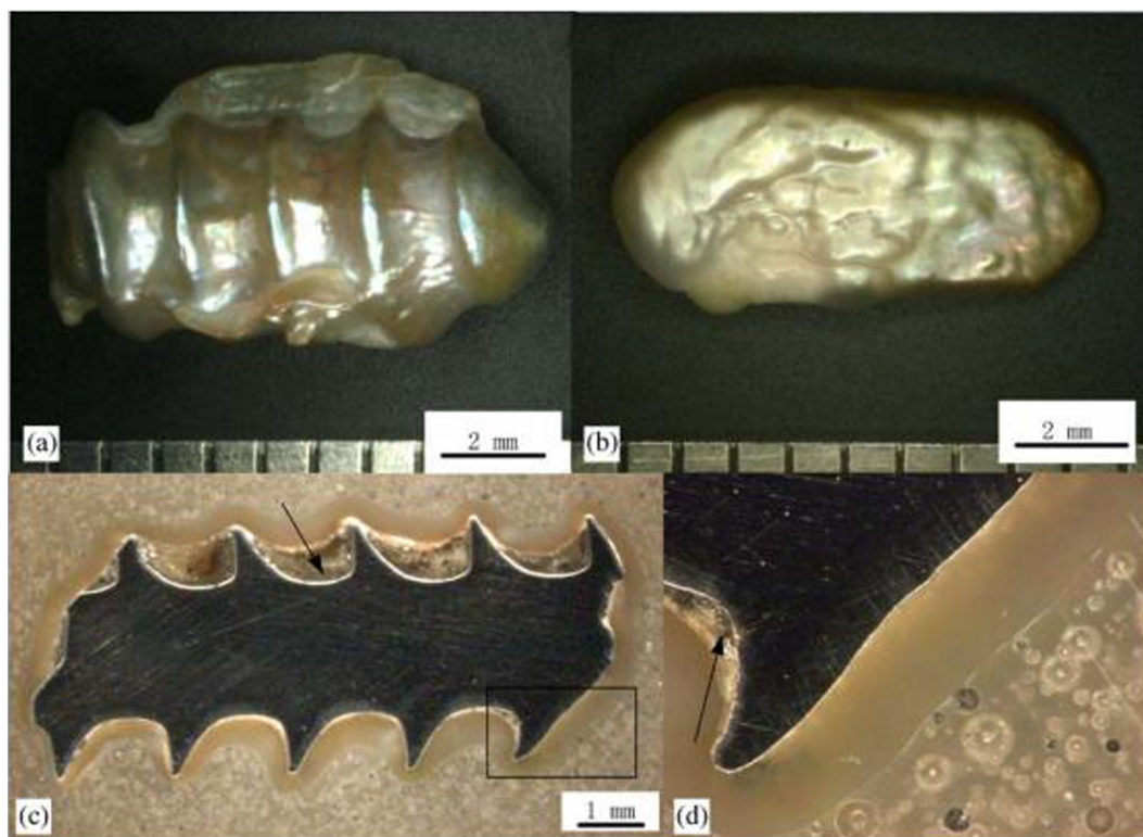
Fig. 5. Biological coating of titanium cultured in pearl sacs for 45 days. (A) and (B) Nacreous coatings on dental implant screws and flat plates respectively. (C) Longitudinal section of coated screw. (D) Enlarged image of selected area from (C) showing the interface between the coating and screw. Reprinted from [148], with permission from Elsevier.
