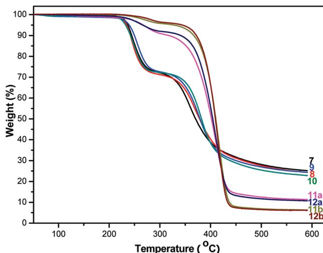
Figure 2. TGA curves of polymers 7–10, 11a, 11b, 12a, and 12b in N<sub>2</sub>.
